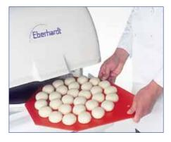
When the **OPTIMAT** has the dough divided and moulded the visor opens automatically and you can take out the moulding plate with the optimally divided and moulded dough pieces on it.
