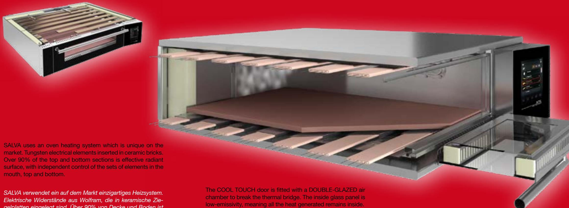
SALVA uses an oven heating system which is unique on the market. Tungsten electrical elements inserted in ceramic bricks. Over 90% of the top and bottom sections is effective radiant surface, with independent control of the sets of elements in the mouth, top and bottom.
